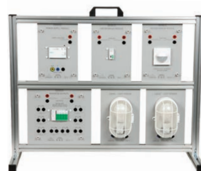
Lighting control study using a presence detector
