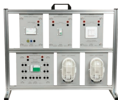
Study of lighting control via push button
