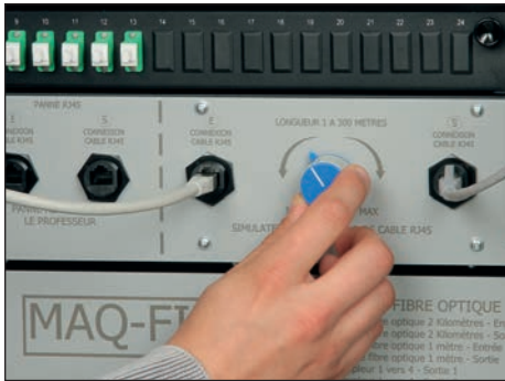
RJ45 cable length simulation potentiometer
