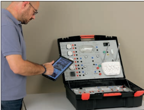
Case with ergonomic handle. Dimensions 534 x 374 x 190mm. Supply by power cord 230V-2P + E.
