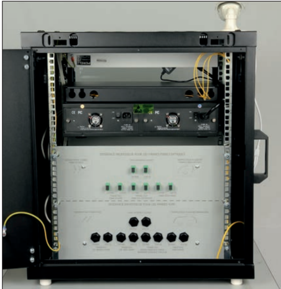
Back side. Teacher interface for fault creation.
