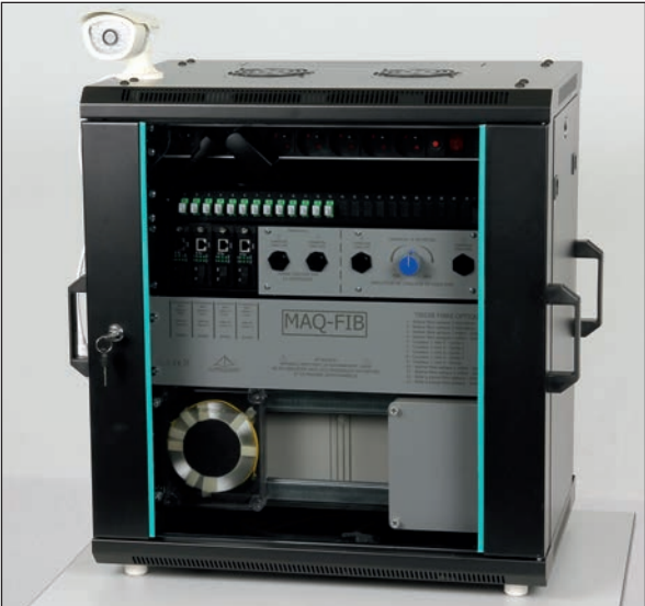
VDI type box with handles (H760mm x W680mm x D450mm) to be placed on table + camera. Weight: 40kg. Power supply by 230Vac power cord of 3 meters (2P + E). Delivered wired and functional.
