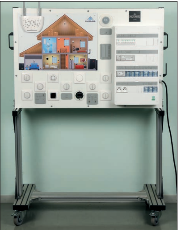
A chassis with wheels in aluminum profile • Dims : (W)1200 x (D)700 x (H)1700mm - Weight: 94 kg ref. MCP-MH-R Version with wheels
