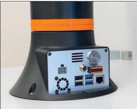
Electronics, power supply and com ports centralized in the robot foot
