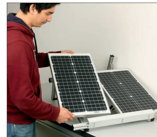
Panel installation: The frame can be tilted to simulate roof installation.
