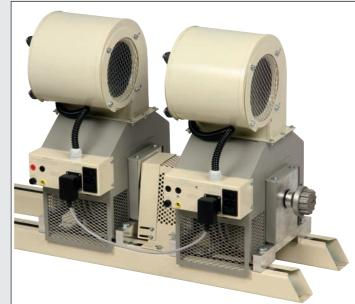
As the powder brakes of the other ranges, a simple DC current under a low voltage around 14V generates a constant braking torque for all the speeds
