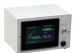
Digital display for the study of rotating machines (from 300 W to 3 kW).
