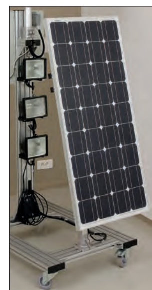
90Wp monocrystalline panel swivel for use interior with the 3 projectors supplied, outdoor with a natural solar source.
