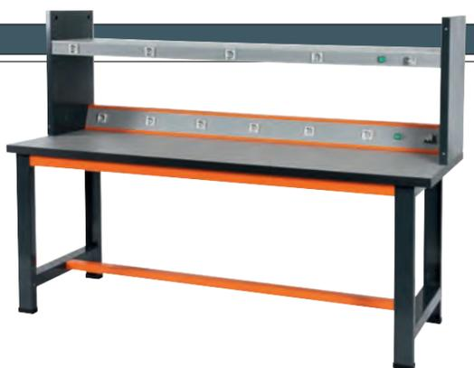
OPTION NAPPE ANTISTATIQUE DISSIPATIVE AVEC CORDON DE TERRE
