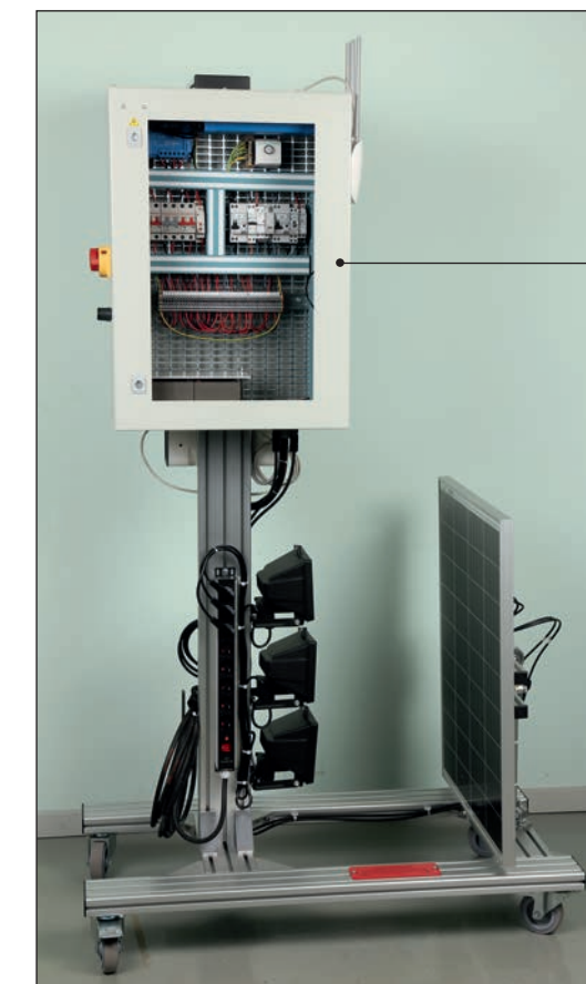
Battery box + charge regulator.
