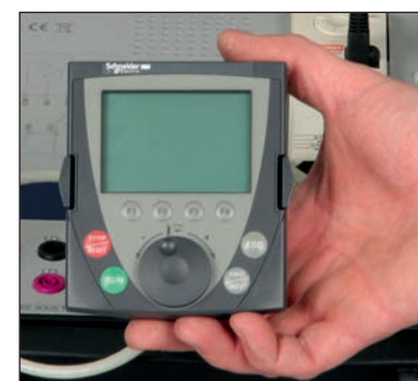
Programming screen of logical inputs/outputs of the variator.
