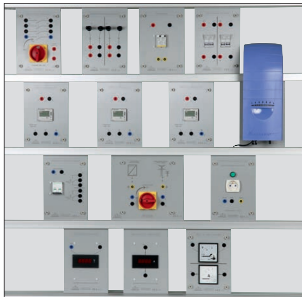
Set of photovoltaic modules (H-250mm) and solar panels for studying a solar installation with energy feeding to the 230V AC grid.
