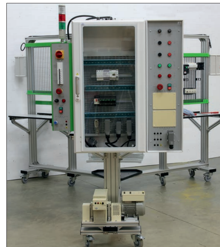
Test cabinet with general power supply console (left), HMI and 300W motor bench console (right)
