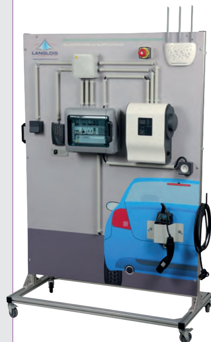
The charging station communicates via Wifi or Bluetooth. The locally created wifi network is specific to the model. It is isolated from the WiFi network of your establishment.
