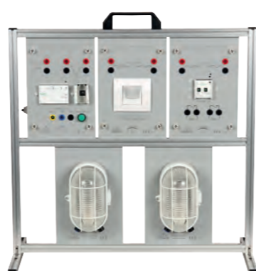
Study of lighting control by presence detector
