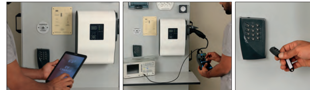
The charging station communicates via Wifi or Bluetooth. The locally created wifi network is specific to the model. It is isolated from the WiFi network of your establishment.
