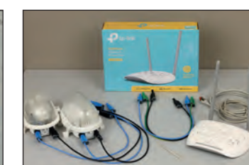
Pushbuttons are easily removable without a tool to facilitate access to the programming buttons.
