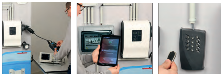
The charging station communicates via Wifi or Bluetooth. The locally created wifi network is specific to the model. It is isolated from the WiFi network of your establishment.
