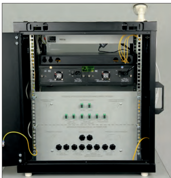
Back side. Teacher interface for fault creation.
