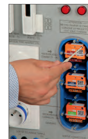
Pushbuttons are easily removable without a tool to facilitate access to the programming buttons.
