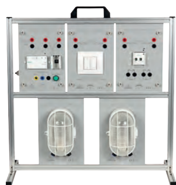
Study of lighting control by pushbutton
