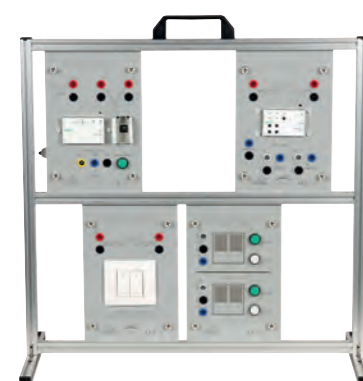
Study of roller blind control by pushbutton
