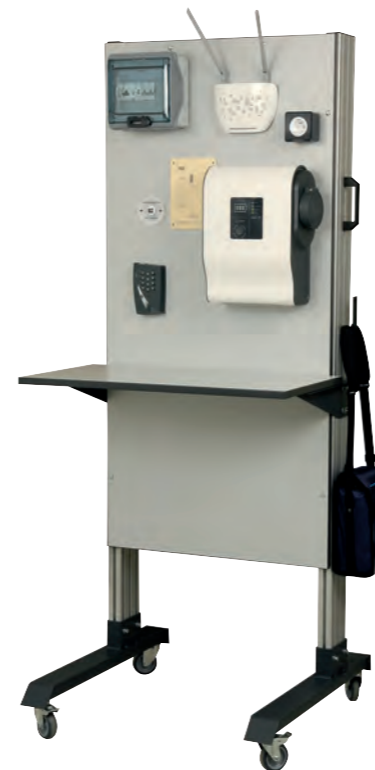
The charging station communicates via Wifi or Bluetooth. The locally created wifi network is specific to the model. It is isolated from the WiFi network of your establishment.
