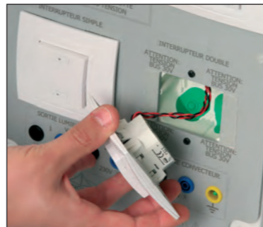
Pushbuttons are easily removable without a tool to facilitate access to the programming buttons.
