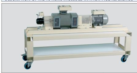
3-phase asynchronous motor Ref. MAS22 - Qty 1 (features P. 54) Rotary torque sensor Ref.CR2-V2 - Qty 1 (features P. 58) 3-phase alternator Ref. MSM20 - Qty 1 (features P. 54) DC tachogenerator Ref. DYTA2 - Qty 1 (features P. 58) Stand on wheels Ref. CTC - Qty 1 (features P. 59) Guide rails Ref. RGC - Qty 1 (features P. 59)
