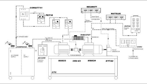
The PACK-AC2 power unit kit (power unit + accessories) can be used for studying a 1500W asynchronous motor.
