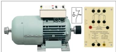
Works as a synchronous motor and a 3-phase alternator. Equipped with LEBLANC poles for mains network synchronization.
