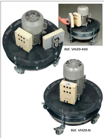
On the base of a propeller fan, a 1500W motor is direct-coupled to the propeller in a 500mm diameter shaft. In this way, this small group forms a dynamic load designed for studying the load currents of a motor.
