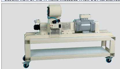
DC motor Ref. CC20 - Qty 1 (Features P. 55) Rotary torque sensor Ref.CR2-V2 - Qté 1
