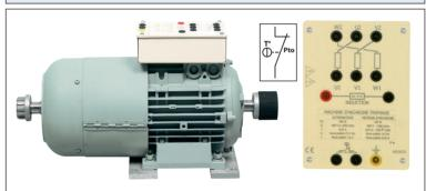
Works as a synchronous motor and 3-phase alternator. Equipped with LEBLANC poles for the mains network synchronization.
