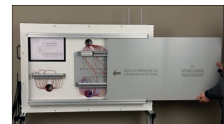
The components are wired on the rear panel via industrial terminals to prevent wear of the component terminals.
