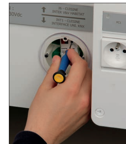
The set of switches of habitat type and KNX are integrated on the front panel. A translucent plate on the universal adapter, covers the connectors and protects electrical contacts, only the programming buttons remain accessible. The push buttons are very easily removable to facilitate access for programming.
