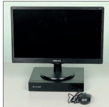
Supplied with an 18" HD LED recorder and monitor representing the security post.
