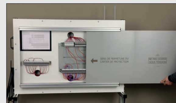
The components are wired on the rear panel using industrial terminals to prevent wear of the component terminals. A housing protects access to industrial terminals during live tests. Removable wiring diagram.
