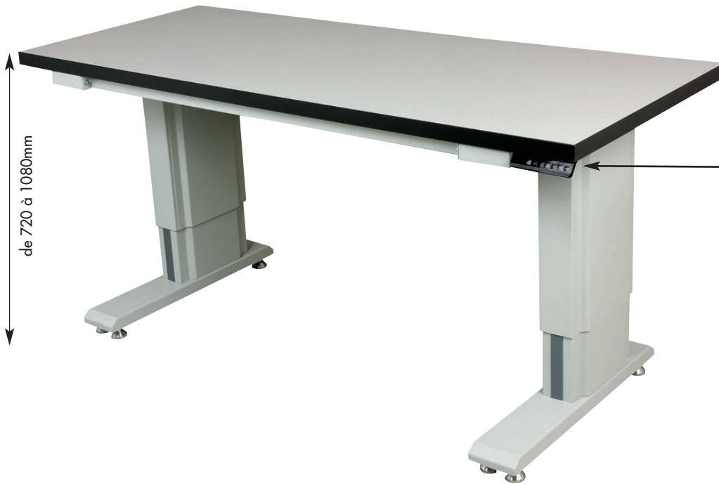
Electric command affixed under the worktop. 4 memorized positions. Digital height display.
