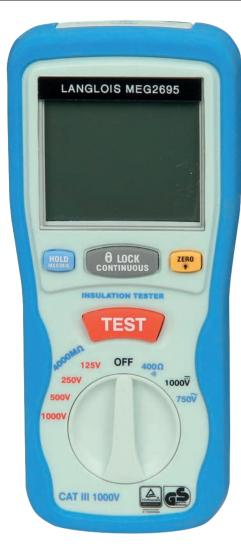
The MEG2695 megohimmeter has 4 measuring functions: insulation resistances with 4 test voltages (125V, 250V, 500V, 1000V), resistors, DC voltage and AC voltage.
